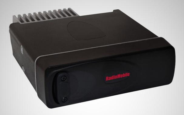
Integrated RF - Transceiver Micro-multiport controller Integrated GPS - option Multispeed: 4.8kb, 9.6kb, 19.2kb, 22kb Speeds up to 48kb capable Modes: mmp 30, 31, RM, serial interface, IP Built-in GPS receiver (as option) VHF, UHF, 700, 800 900 MHz Industry competitive performance Variable power; options up to 35 Watt UHF and 800 Mhz - 50 Watt up to 110 Watt VHF
