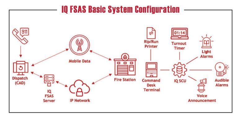
The CAD can communicate with the fire stations over traditional RF networks or over wired or wireless IP networks. The IQ FSAS Server provides an IP interface to the CAD and relays dispatch messages and status updates between the CAD and the fire station, specifically the Command Desk Terminal and the IQ Station Control Unit. These, in turn, control the peripherals including lights, speakers, turnout timers, bay doors and other equipment.
